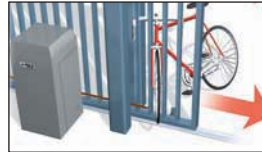
entrapment prevention system reverses gate on contact
